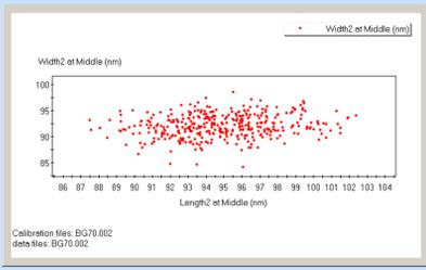
Fig. 7. Scatter plot of Width vs. Length and Width of bumps. Each point represents one bump. Feature length varied from 88 to 102 nm and width ranged from 84 to 94 nm. There was no apparent correlation between length and width.
