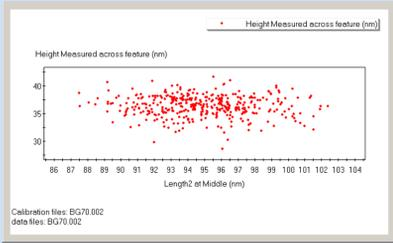
Fig. 8. Graph of height vs length. Height is measured between the top of the bump and the land to the side (direction parallel to the X axis in the image). There was no significant correlation between these two parameters.
