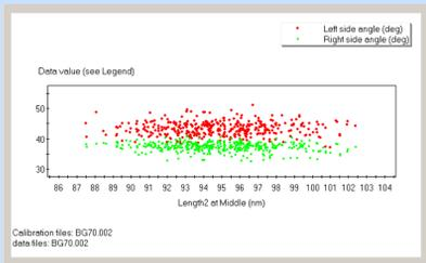
Fig. 10. This chart directly shows that the side wall angles did not correlate with bump length, remaining relatively constant over the range of feature lengths.
