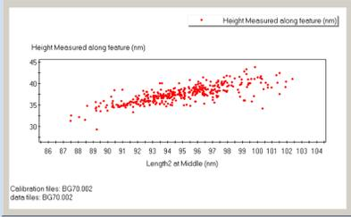
Fig. 9. In this chart the height is measured between the top of the bump and the land either in front of or behind it (parallel to the Y direction in the image). The longer bumps tended to be taller. A similar chart (not shown) showed a correlation between height measured across the bump and the bump width. These correlations indicate that the side and end wall angles did not change noticeably with bump size.
