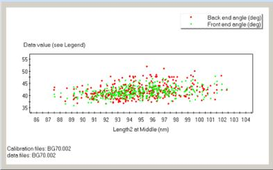
Fig. 11. As with left and right angles, the front and back angles remained approximately constant with feature length, or perhaps increased slightly. This slight correlation is probably not significant.
