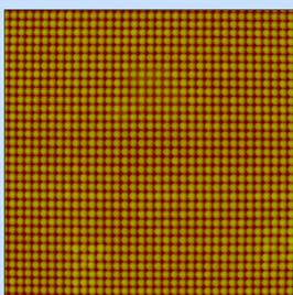
Fig. 3 Test sample: 144-nm pitch, 2-D holographic grating of Al bumps on Si. Mean pitch of X axis =  $143.928 \pm 0.015$  nm (measured at PTB)
