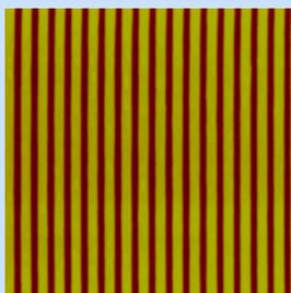
Fig. 2 Calibration standard: 292-nm pitch, 1-D holographic grating of Ti lines on Si. Mean pitch =  $292.096 \pm 0.015$ nm (measured at PTB)
