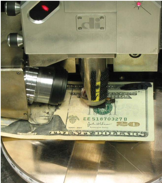
Fig. 2 Dimension 3100 AFM at ASM showing the scanner and a large test specimen.
